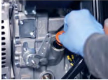
**2.** To check the oil in a standard Redbox generator, remove the dipstick with the orange cap located in the side of the engine. Check that the oil level is between the MIN and MAX markers on the dipstick.
