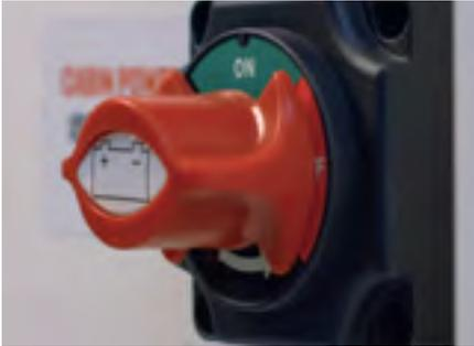
**1.** Before starting the generator, turn the Cabin Power Isolator switch in the cabin to the ON position.
