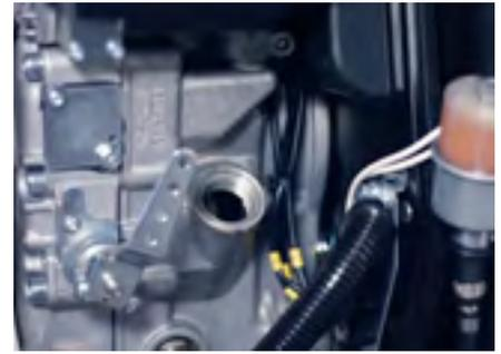
**3.** If your generator needs more oil, fill with suitable engine oil through the same hole as the dipstick is located. Be careful not to overfill, only fill up to the MAX level on the dipstick. Always use the grade of oil specified in the appropriate RedBox generator manual.
