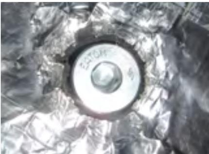
Before towing the unit any water in the clean water tank must be removed. The drain for the clean water tank is located on the underside of the trailer towards the rear, beneath the toilet compartment.
