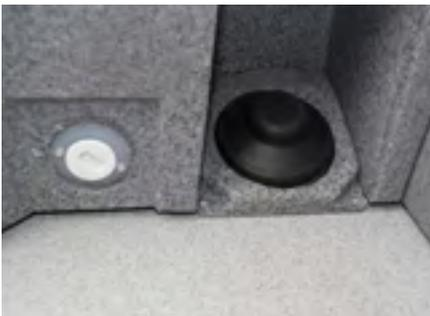
Before towing the unit, any water in the clean water tank must be removed. There are two ways to drain the tank. Either by depressing the foot pedal and running all water out of the reservoir into the sink from which it will move to the waste tank. Or you can remove the white drain plug from the base of the sink and the water will run out from there.
