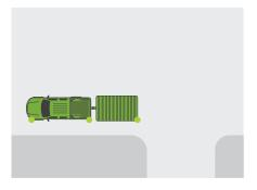
1) Position the towing vehicle parallel to the kerb and if conditions allow, approximately 1m to 1.5m from it.
