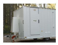
**1.** To attach your cabin to a towing vehicle it should be in a raised position with wheels on the floor and rams raised. See Manual Section 3.1 for instructions.
