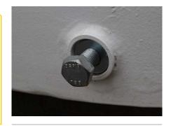
**1.** First remove the plugging bolt from the eye hole.
