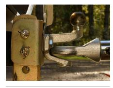
**3.** Manoeuvre the towing vehicle so the coupling eye is aligned.
