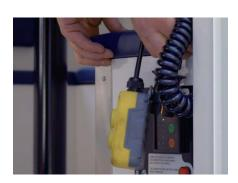
**13.** Unplug the remote control unit and stow it safely inside the bench in the cabin for road use.
