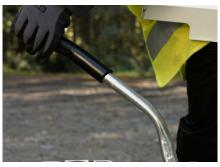
**2.** To uncouple the unit from the towing vehicle, first apply the parking brake.
