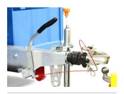
**3.** Turn the Jockey wheel operating handle anti-clockwise to raise the coupling head higher than the towing vehicle's tow ball. Then manoeuvre the towing vehicle so the ball is beneath the ball coupler.
