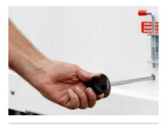
**6B.** (Double Axle Version) Locate the two axle handles on the side of the cabin. Lift the spring bolt into the open position, then pull out the handle to release the axle locking mechanism. Repeat for both axles.
