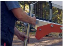
**8.** Pull the handle and rotate the jockey wheel assembly into the down position.
