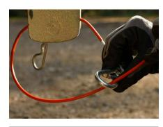
**6.** Attach the breakaway cable to tow hitch of the towing vehicle and ensure it is safe and operational.
