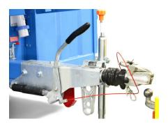
**9.** Keep turning until the hitch is raised above the ball and the towing vehicle can be removed easily.
