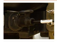
**7.** Connect the lighting cable plug to the socket of the towing vehicle and ensure all lights are functioning correctly.
