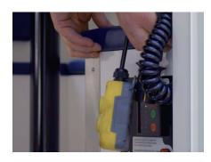
**11.** Unplug the remote control unit and stow it safely inside the bench in the cabin for road use.
