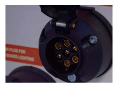
**6.** Remove the remote control from its storage position inside the bench behind the generator and connect the remote control's 7 pin plug to the correct socket on the front of the unit.
