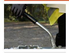
**4.** Raise the parking brake lever to engage the brake.
