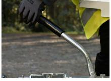
**2.** With the unit positioned on level ground apply the parking brake by raising the lever.
