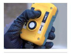
**7.** Press the black RAISE button on the remote control to extend the ram cylinders to raise the cabin until the wheels are clear of the ground.
