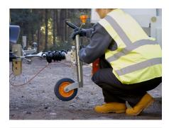
**4.** Rotate the jockey wheel assembly through 90 degrees anti-clockwise into down position.
