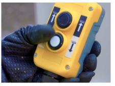
**11.** Ensure there are no obstructions beneath the unit, then press the white LOWER button on the remote control to retract the rams and lower the unit onto the road wheels and jockey wheel.
