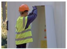
**2.** Raise the anti-vandal cover into the towing position.
