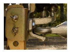
9. Remove the coupling pin.
