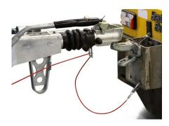
**7.** Detach the breakaway cable from the tow hitch of the towing vehicle.
