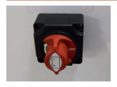
**12.** Turn the Cabin Power Isolator switch in the cabin to the OFF position.
