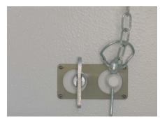
**3.** Then engage the anti-loose fastener and the safety pin to ensure the cover stays in the towing position when on the road.
