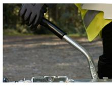
**2.** With the unit positioned on level ground apply the parking brake by raising the lever.
