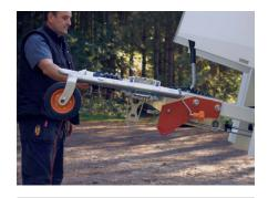
**10.** Stand clear of the drawbar and jockey wheel assembly as the unit is lowered to the ground.
