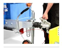
**4.** Raise and hold the coupling head handle in the up position, and then turn the jockey wheel clockwise to lower the coupling onto the tow ball.
