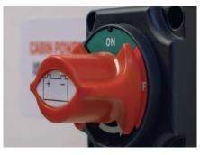
**5.** Turn on the Cabin Power Isolator switch inside the cabin.
