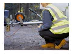
**10.** Rotate the jockey wheel assembly through 90 degrees clockwise into locked position.
