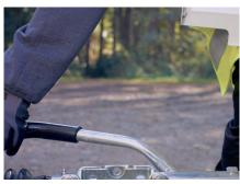
**10.** Release the unit's parking brake by lowering the lever.
