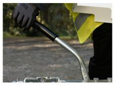
**11.** Release the unit's parking brake before towing by lowering the lever.
