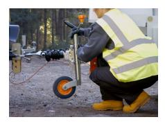
**4.** Rotate the jockey wheel assembly through 90 degrees anti-clockwise into down position.
