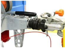
5. When almost fully lowered let go of the coupling head handle and allow it to snap closed over the tow ball. Check that the coupling head is fully engaged on the tow ball.
