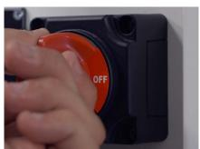
**14.** Turn the Cabin Power Isolator switch in the cabin to the OFF position.
