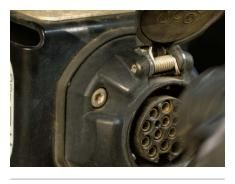
**6.** Disconnect the lighting cable plug from the socket on the towing vehicle.
