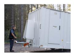
**9.** Continue to press the LOWER button until the ram cylinders have fully retracted and the unit is lowered to the ground.
