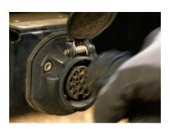
**6.** Disconnect the lighting cable plug from the socket on the towing vehicle.
