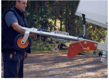
**7.** Stand clear of the drawbar and jockey wheel assembly as the unit is lowered to the ground.
