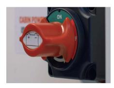
**3.** Turn on the Cabin Power Isolator switch inside the cabin.
