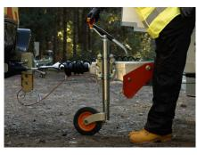
**5.** Then turn the jockey wheel operating handle anti-clockwise to lower the jockey wheel to the ground.
