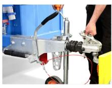
**8.** Lift the handle behind the tow hitch to release the ball hitch from the towing ball. At the same time turn the jockey wheel handle anti-clockwise.
