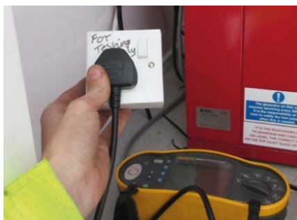
The test equipment plugged into generator using adaptor
